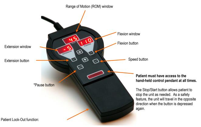
The lock-out switch is located on the back of the control pendant under the plastic door cover. To prevent inadvertent changes to pendant settings, simply slide the switch to the locked position. The ROM window will read 'LOC' should attempt be made to adjust settings when this is in place. The stop/start button functionality remains the same.
